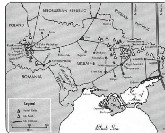
Figure 6.4 Map of gas fields and long-distance gas pipelines in the Ukrainian SSR as of the late 1960s. Before eastern and western Ukraine were more tightly interlinked, all Soviet exports of natural gas depended on deliveries from Galicia's (western Ukraine's) gas fields, here shown to the left.
